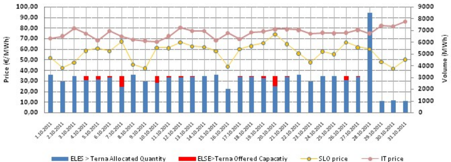
Correlation between offered and allocated quantity of daily capacity on SI- IT border and difference between Base price on SI and IT market
